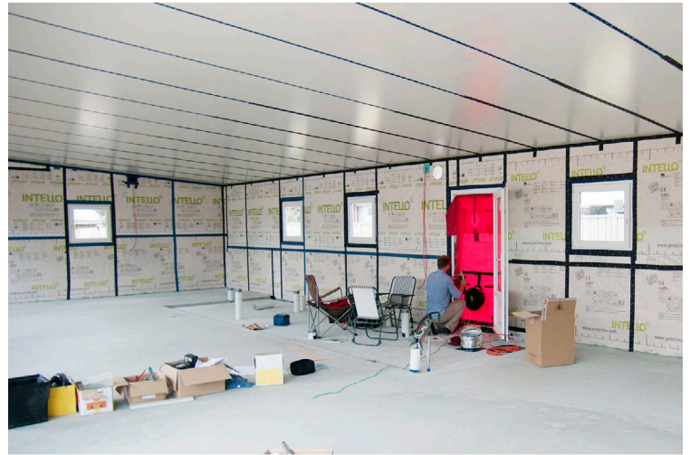
↑ Blower door testing ascertains envelope airtightness by sucking internal air out through the door and testing for any air infiltration into the building through gaps.
